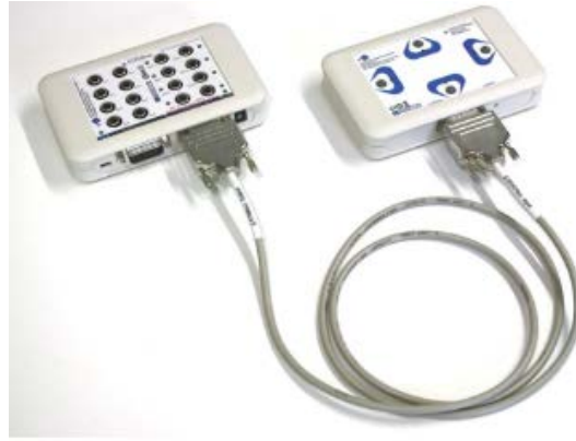
Figure 26. The SSVEP stimulation-box (g.tec, 2013).
